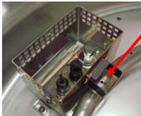
Pilot Window lined up with burner hole.
